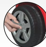
Push button wheel release
