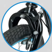
Front and rear caliper brakes
