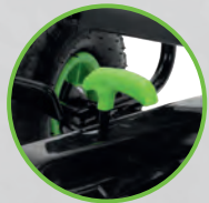
Freewheel gear for coasting
